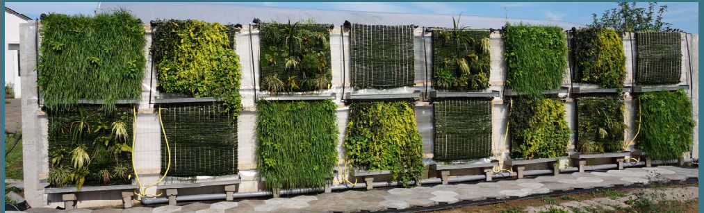
fig.2: One Experimental wall, exposed to west, with the variants: sowing, cascade, ground cover and control (without plants); closed irrigation system with nutrient solution stored in a cistern
